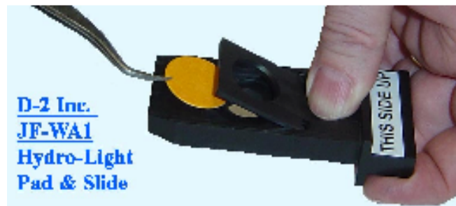
Inserting the Water Pad into the Pad Holder with Tweezers.
